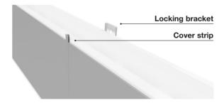
Locking bracket between each element on the **RE60** hight, otherwise if needed.
