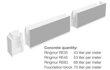
Fill concrete in the blocks by walk around two rounds. If you also have foundation block three times is needed. Use reduced speed on concrete pump and do not use vibrator. Put the top reforcement in at the end and make a smooth surface on concrete. Concrete prescription is B30 with D-max 16 mm, 25 % reduced content of gravel, slump test level 16-18 cm.
